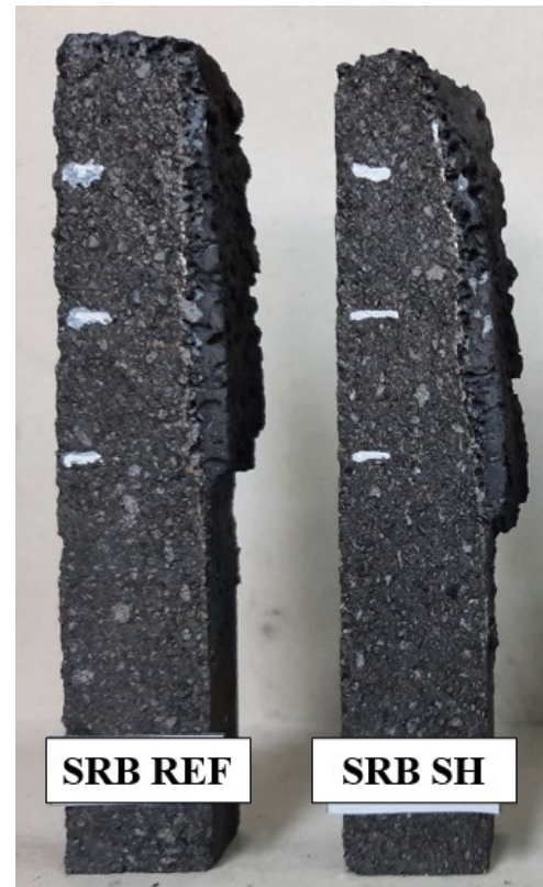
Fig. 7. Cross-section of SRB REF and SRB SH samples after the corrosion test.
